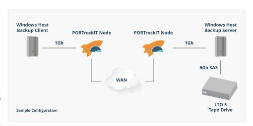
Companies often try to solve TCP/IP performance issues by investing in more expensive network infrastructure that offers a larger maximum bandwidth. However, this does not fix the underlying problem of latency. Latency and packet loss prevent TCP/IP connections from fully utilising the available bandwidth - so any extra investment in bandwidth will simply be wasted unless the latency and packet-loss issues can be addressed.
